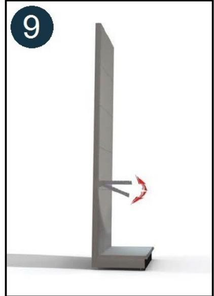
Rotate the bracket upwards until secured in a horizontal position. Brackets can also be positioned at sloping angles if desired.
