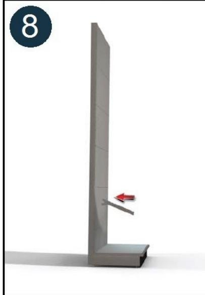
Insert a bracket into the upright "H" slot at an angle as shown above.
